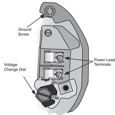
**Figure 7: Voltage set to 230 volts, Dial Type**
