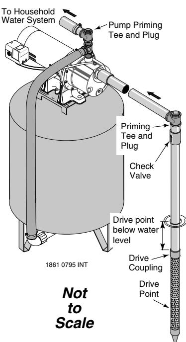
**Figure 1: Driven Point Installation**
