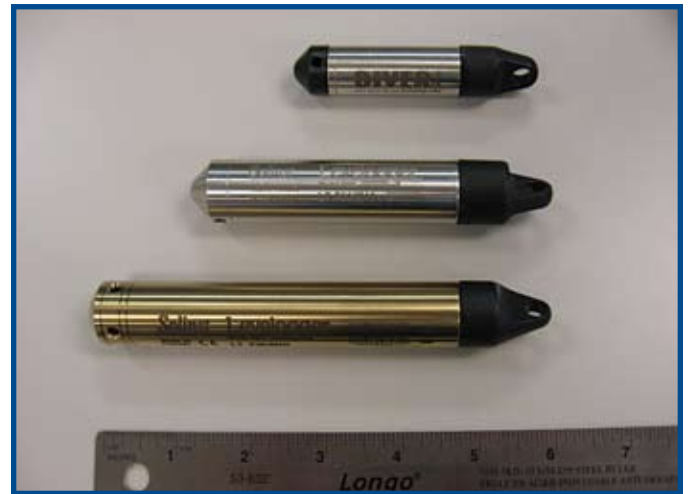
Figure 7. A pressure transducer can be used for automatic measurement and recording of water level and temperature, specific conductance or other parameters during the pumping test.
