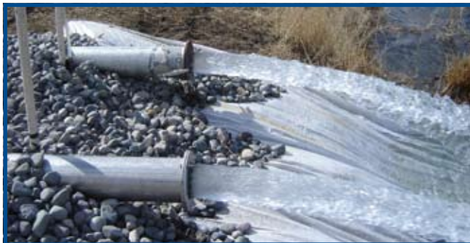
Figure 3. Water discharge during a pumping test
