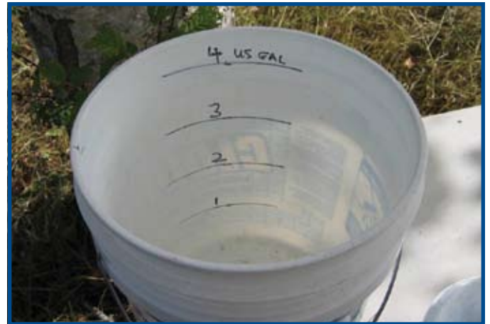
Figure 5. A five gallon bucket (~20 liters) and a stop watch can be used to estimate low pumping rates.
